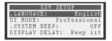
The S8000/S4000 Pro has many global parameters that users can check or configure. Users access these through the settings options in the Global Settings View (GSV). These global parameters may relate to the entire charger, a specific channel, or certain programs. Changes to the settings are not saved until a depress of ENTER (= save and exit) exits the view.
