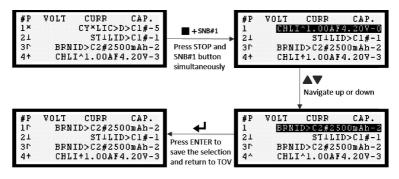
8. Copy Operation, This operation allows users to quickly copy a channel's program to other inactive channels in Normal and Professional Modes. In this example, all four channels are inactive, and we will copy Channel 1's program to Channels 2, 3, and 4: Step 1: Simultaneously press SNB#1 and SNB#4. This will activate the copy operation for all inactive channels between the two selected channels.
